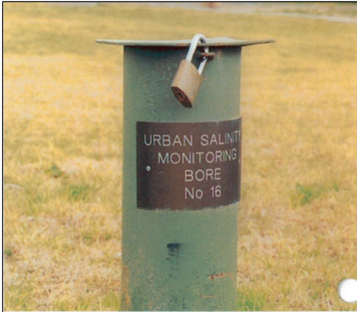
Figure 1: Piezometer, image from Broadsheet: Urban Salinity in Wagga Wagga
